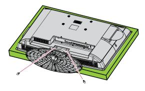
3 Attach the wall-mount bracket to your TV/DVD combo using the mounting holes on the back of your TV/DVD combo. See the instructions that came with the wall-mount bracket for information about how to correctly hang your TV/DVD combo.
